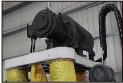
水冷双电机 ( 选配Alternative ) water-cooling of double motor
