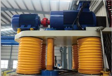
双电机驱动装置 Moved by dual motors
